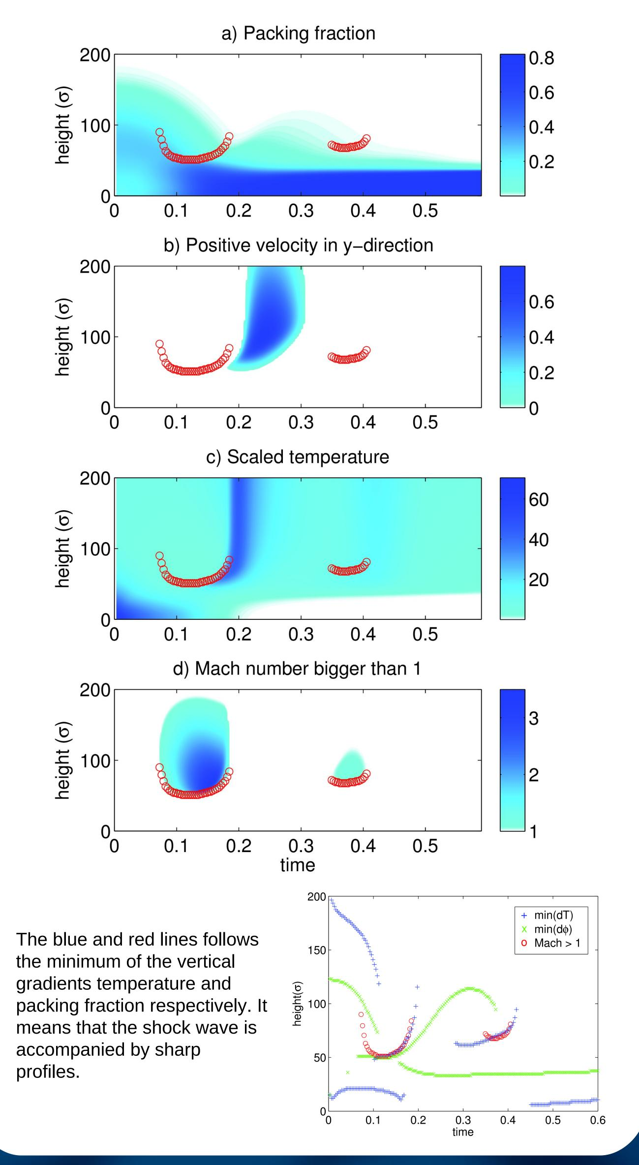
The Navier-Stokes terms are treated by centered high-order explicit in time finite difference approximations and considered as sources for the method of lines in the time approximation. The Euler terms are solved in local coordinates by a fifth-order explicit in time finite difference characteristic-wise WENO method. Complete details on the numerical scheme [2].
