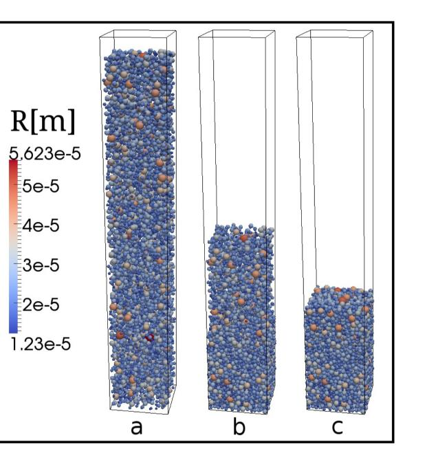
Model 2: viscoelastic forces and adhesion (modeled through JKR theory); Model 3: viscoelastic, adhesion and non-bonded van der Waals forces.
