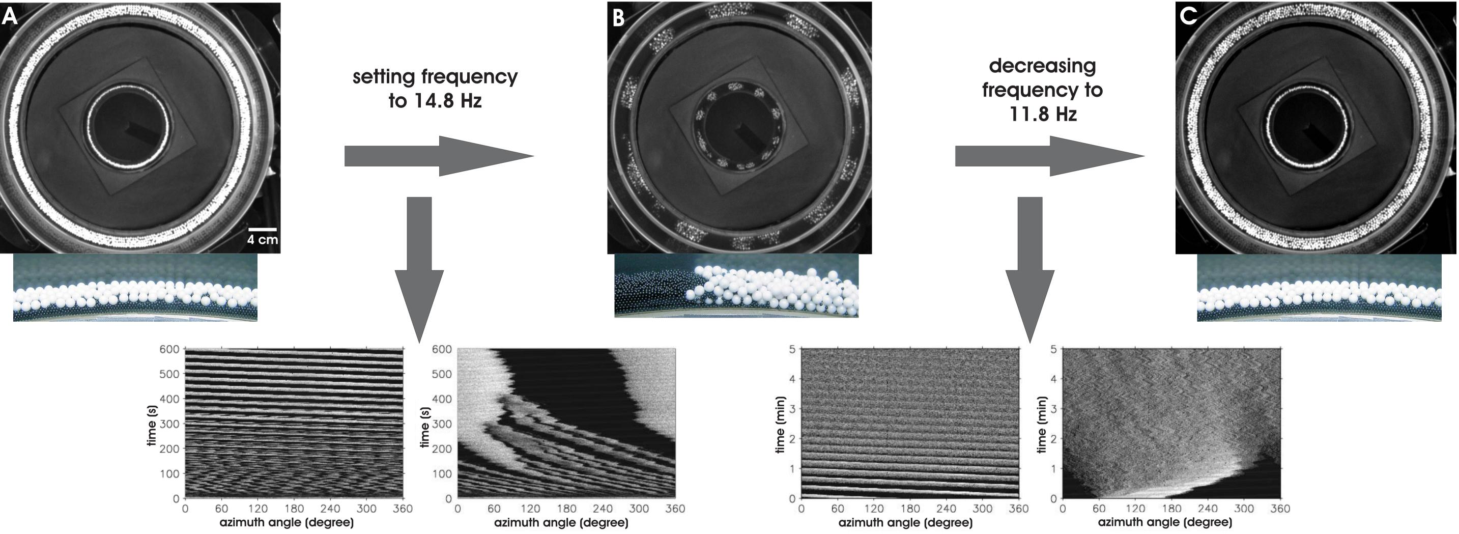
Space-time plots visualize the progress of the lateral segregation and the mixture of the granulate. On each right side you see the segregation and mixture in the granulate system (obtained by 2d Fourier transformation).
