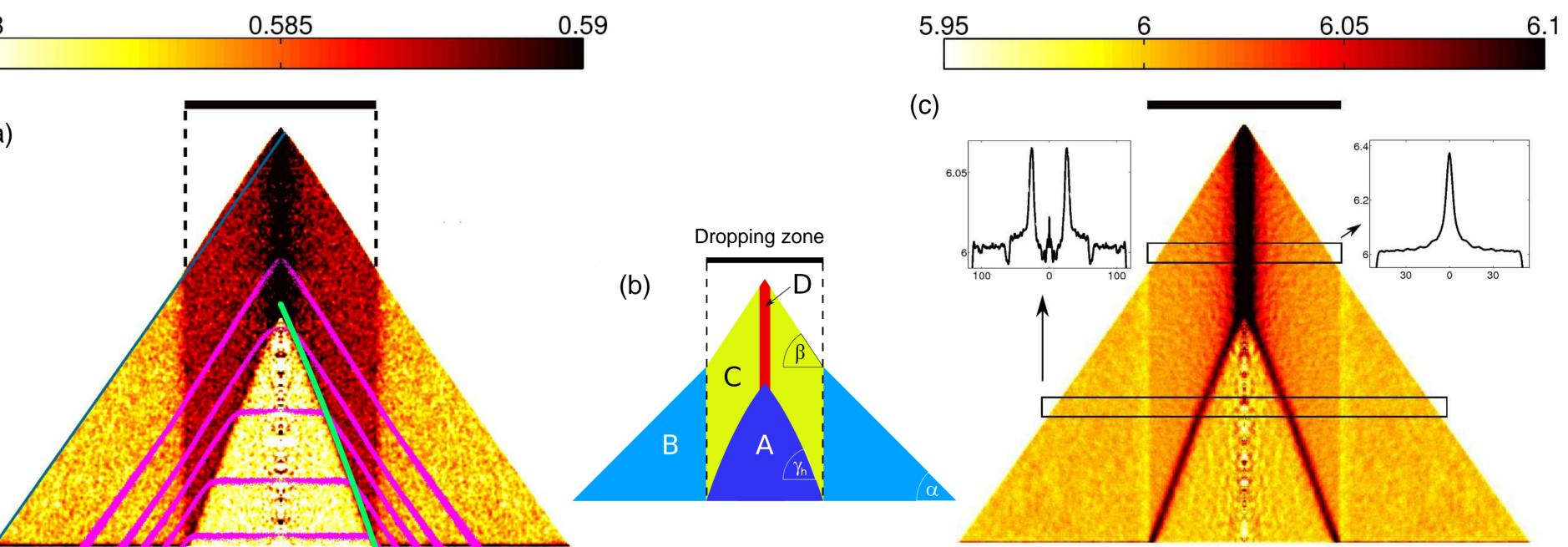
particles,  $N = 10^7$ , deposited from an area source. The yellow and blue lines help the visualisation of two angles of repose
