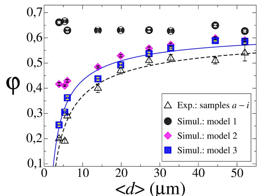
**Fig. 3** – Packing fraction as a function of the average particle size. Empty and filled symbols denote results from experiments and simulations using models 1 – 3, respectively. The best fit to the experimental data obtained using Eq. (1) yields  $C \approx 1.05$  and  $\alpha \approx 0.59$  (dashed line). The continuous line denotes the best fit to the simulation data obtained with model 3, which gives  $C \approx 0.99$  and  $\alpha \approx 0.68$ .
