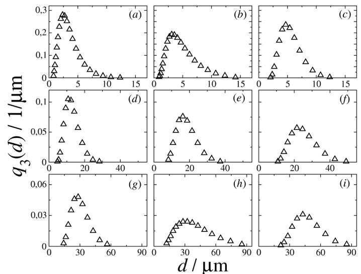
**Fig. 1** – Experimental particle size distributions. In each plot, the volume density distribution is shown as a function of the particle size.
